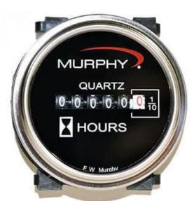
The TM Series hourmeters record the operating time of vehicles or powered equipment. They are electromechanical and have a quartz base time counter that insures accuracy (better than ±0.02% over the entire range). They can record up to 99,999.9 hours (9,999.9 for TM612/624) and include an automatic recycle to zero hours feature.
