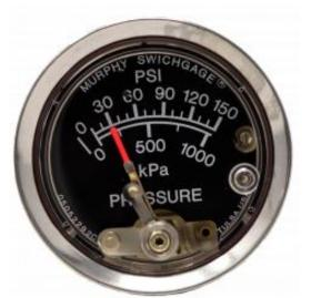
Ranges are available from 0-15 psi (103 kPa) [1.0 bar] through 0-100 psi (690 kPa) [7.0 bar].
