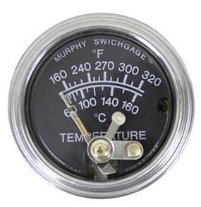
New MURPHY Swichgage model 10-35-0949 fluid temperature gauge with high limit switch. Can be used with coolant, oil, diesel fuel or hydraulic fluid. 1/16" Hex wrench adjustment knob on front to adjust switch set point
