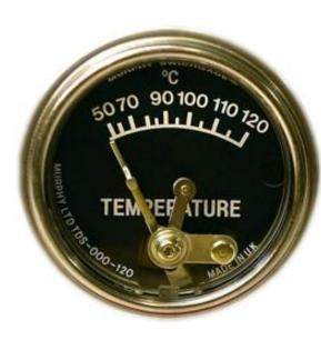
The 20 Series (2 inch/51 mm dial) and the 25 Series (2-1/2 inch/64 mm dial) Swichgage models are diaphragm-actuated, temperature-indicating gages with built-in electrical switches for tripping alarms and/or shut-down devices.
